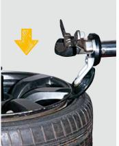
✓ Hydraulic lower bead breaking operation: a second independent but specular disc rises and the wheel performs a specific movement to facilitate the bead breaking operation with a controlled penetration path.
