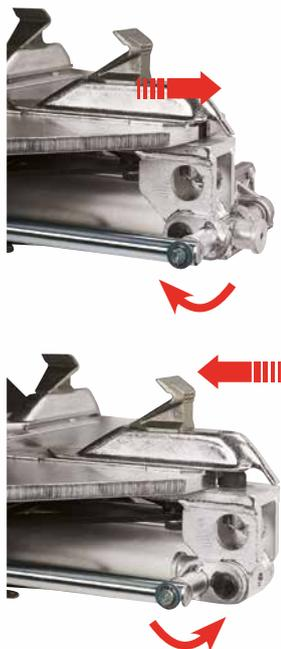
The **AS 946** has a new-concept turntable with mechanism designed to assure high performance over time. **In spite of the breadth of its working range (10"- 28")**, the turntable is compact and has 2 working positions: the first from 10" to 25", the second from 14" to 28".
