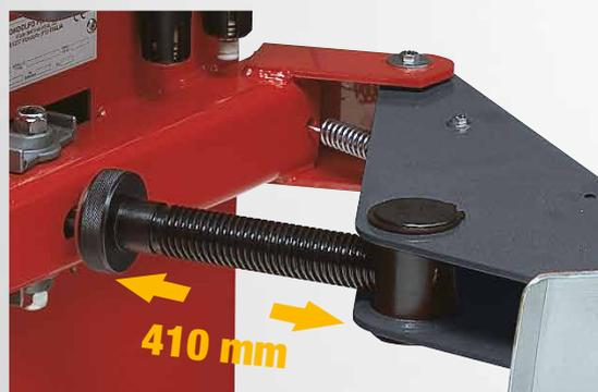
The bead breaker is operated by a double-acting pneumatic cylinder made from 100% stainless steel, generating a power of **15500 N** on the blade.
