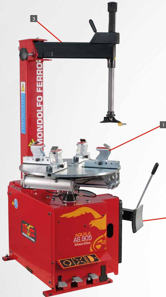
Great attention has been paid to the wheel clamping system. Both standard and special jaws allow correct clamping and protection of the rim profile.
